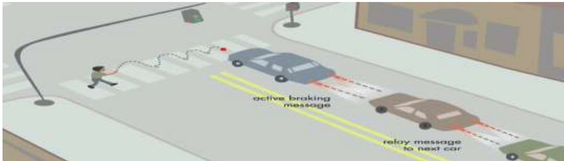
Figure3.Safety application (i.e., brake messaging) by the use of Visible Lighting Communications (VLC)s[21]
